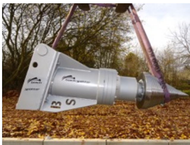
Black Splitter machine lifted with hoisting straps
